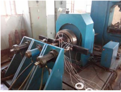
图3 直升机自动倾斜器轴承故障诊断试验系统 Fig. 3 Fault diagnosis test system of helicopter swash-plate bearing
